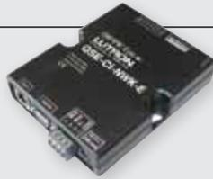
**RS-232/Ethernet interface** allows for seamless integration with A/V, HVAC and building management systems
