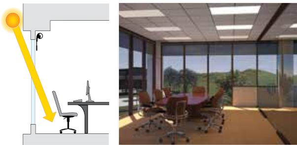
Hyperion software automatically positions shades to let useful daylight into the space. Lights near windows dim to save energy.
